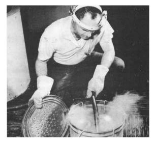
Removal of the alloy is accomplished here by steam line discharging into an odinary steel bucket- Removal could also be done by hot water bath. Individual parts come clean, with only slight hand scouring in the case of anodized aluminum rotors. Lighter metal chips float on molten alloy which is then reclaimed for reuse.
